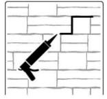
caulking method is to apply or inject the caulk as deep into the gaps so that it has the ability stretch with the expansion and contraction. (see figure 17C). However, in order for the caulked seams to blend in properly it is important not to add too much caulk that draws attention to the joints.
