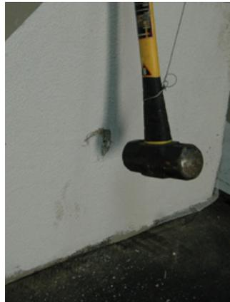
This system is based on 1-3” eps foam / a cement scratch coat/ fiberglass scrim– and finally a textured paint finish.
