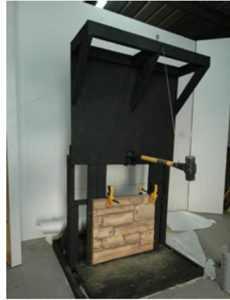
After 3 full hits, the hammer bounced off the panel and did not cause any damage to the panel
